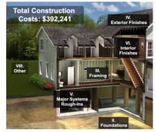
construction costs into 8 major construction stages. Interior finishes, at 24.0%, accounted for the largest share of construction costs, followed by framing (20.5%), major system rough-ins (17.9%), exterior finishes (11.8%), foundations (11.0%), site work (7.4%), final steps (5.9%), and other costs (1.5%).
